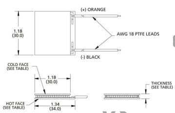
Ceramic Material: Alumina (Al<sub>2</sub>O<sub>3</sub>) Solder Construction: 271°C, Proprietar
