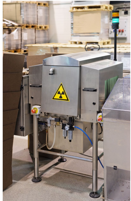
X-ray scanning equipment is often used for quality control in food processing plants.
