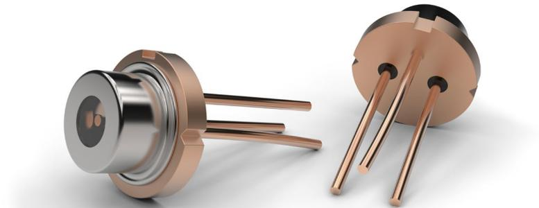
*Laser diodes enable fast data transmission at very far distances
