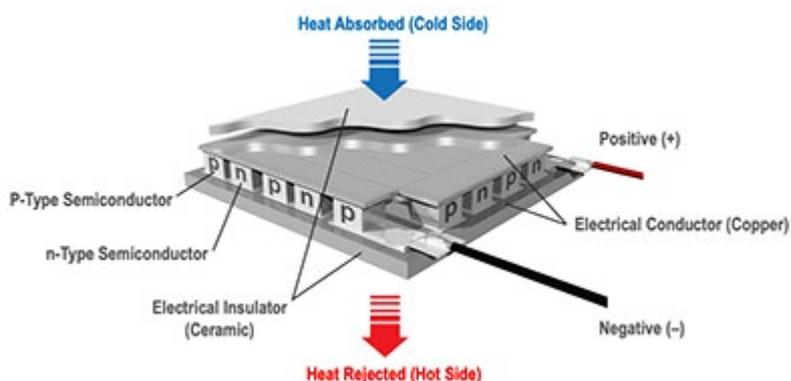
*Thermoelectric coolers remove heat by utilizing the Peltier Effect.*
