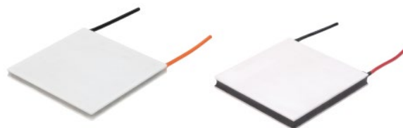
Thermoelectric Coolers used in HPLC equipment are typically sealed with Epoxy (left image) or RTV (right image) in order to prevent moisture intrusion.
